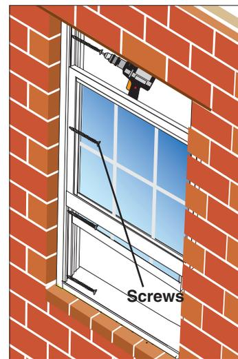
**Wood Bucks must be anchored to openings with the same spacing as used in laboratory tests. Window anchors, direct to the opening or to an installed buck must also match the spacing used in laboratory tests.**
