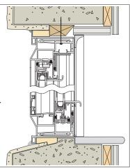
NOTE: Drawings are not necessarily to scale or representative of any particular window type or opening. They are for guidance. Actual situations and products may vary. Quality Sealants and Low Expansion gunnable Foam can be used where indicated to seal against water penetration and insulate against air and moisture penetration as long as the 5 Barriers are properly reconstructed and reconnected.
