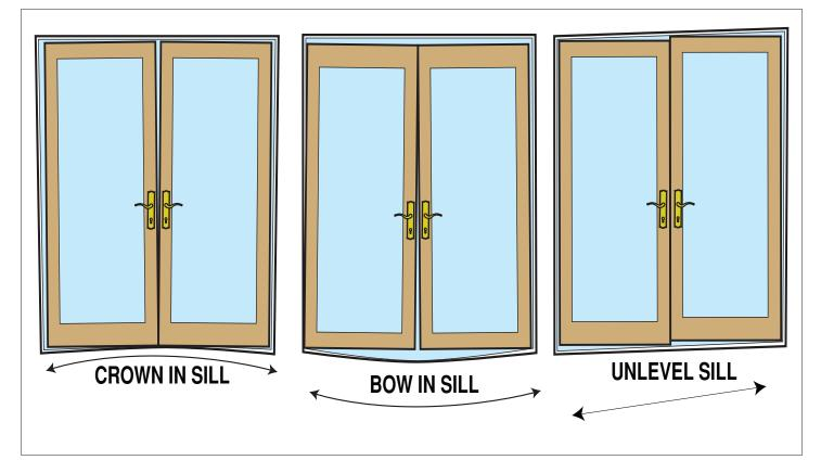
barrier and siding is key. In replacement, as the photos illustrate, removing an old door can either destroy the integrity of the old sill, or expose the fact that there was no integrity in the first place. Filling the old sub sill with mortar or even the same thin set as used with tiling floors, can create the sealed, level and strong sub sill a successful door installation requires.
