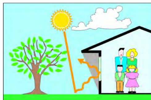
that radiate multi-directional heat waves that would enter the home through the windows, even long after the sun has set. Low "E" prevents the passage of this re-radiated heat into the home, keeping it cooler.
