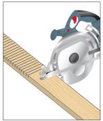
Kerfing - cutting multi grooves in wood to facilitate bending
