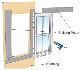
mounted, run a bead of caulk around the inside of the fin.
