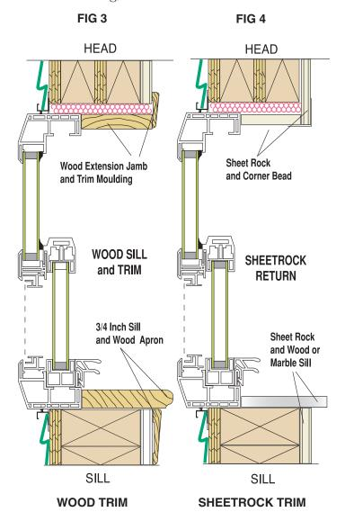
Figure 3 details typical, conventional wood trim - including wood jambs, wood stool, and clamshell or colonial casing and apron. Using standard 3/4" or 5/4" wood stock, butt the stool and jamb to the window, and then the sheetrock can be butted to the jamb and stool and covered as shown.
