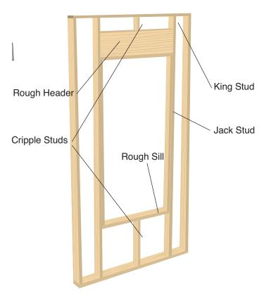
The rough opening should look similar to Figure 1. No window should be installed without a proper header and sill support. All framing should be in compliance with local codes.
