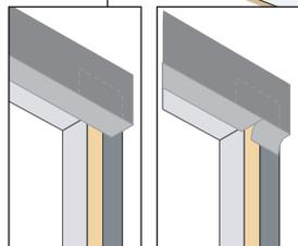
Simplex Cap Nails OVER fin allows frame to move better than nails through mounting slots
