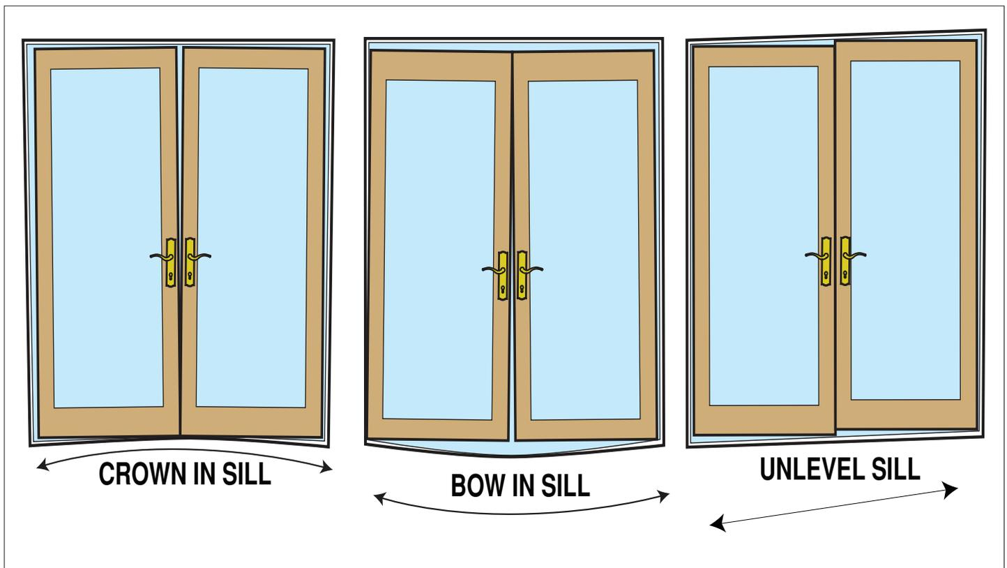
barrier and siding is key. In replacement, as the photos illustrate, removing an old door can either destroy the integrity of the old sill, or expose the fact that there was no integrity in the first place. Filling the old sub sill with mortar or even the same thin set as used with tiling floors, can create the sealed, level and strong sub sill a successful door installation requires.
