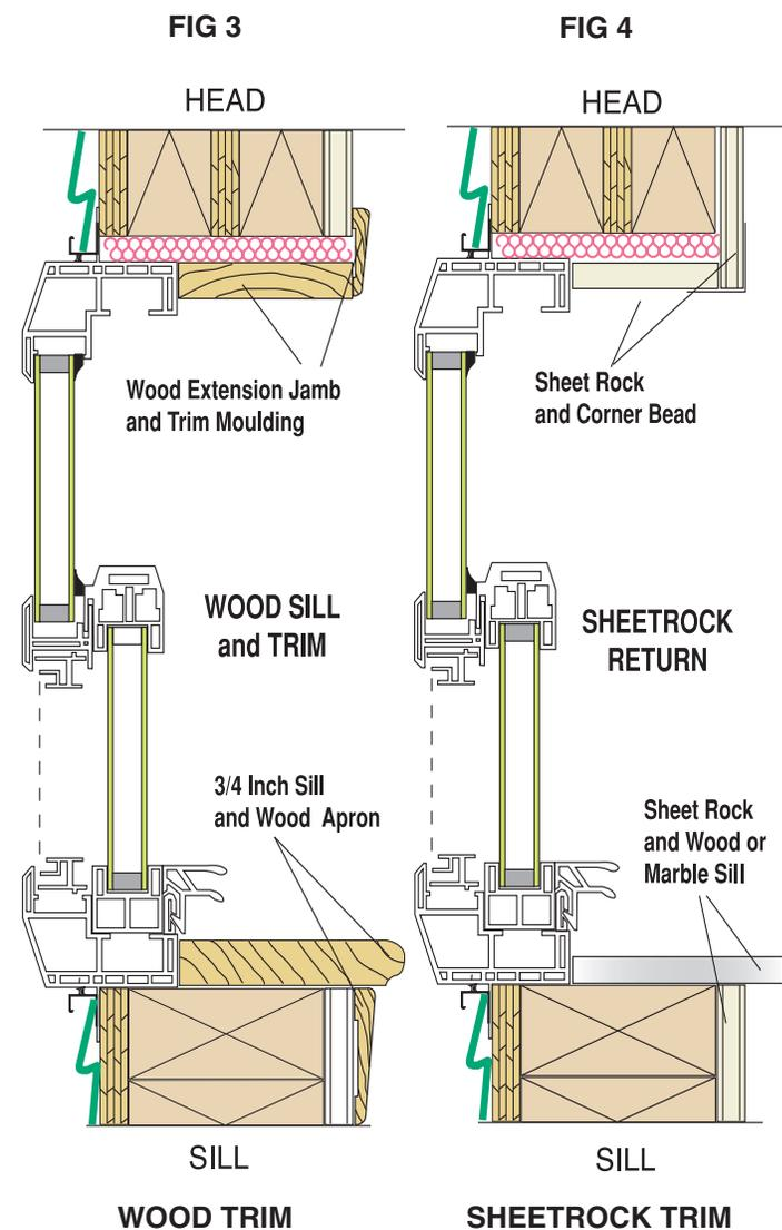
Figure 3 details typical, conventional wood trim - including wood jambs, wood stool, and clamshell or colonial casing and apron. Using standard 3/4" or 5/4" wood stock, butt the stool and jamb to the window, and then the sheetrock can be butted to the jamb and stool and covered as shown.
