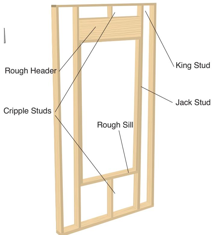
The rough opening should look similar to Figure 1. No window should be installed without a proper header and sill support. All framing should be in compliance with local codes.
