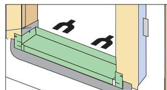
**Caulking and Sealing:** The best sealant is silicone-based or urethane-based to be sure that it adheres to the two materials being sealed. Joints greater than 1/8" to 1/4" should contain backer rod to maintain the bond during expected expansion and contraction of the materials. All mounting holes should be caulked over, and the top edge of the sill pan be sealed before the adhesive backed flashing is placed over the pan and it's mounting nail head.
